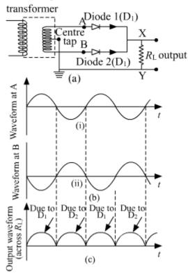
(a) Full wave rectifier circuit
