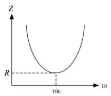
Here,  $\omega_0$  represents the resonance frequency for the LCR circuit and *R* is the resistance of the circuit.
